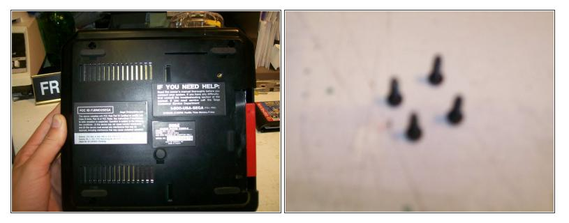
Next, remove the four, black 11mm screws from the bottom of your console.
