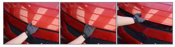
• Raise the hood by simultaneously lifting and pressing up on the hood latch release (usually located beneath the front edge of the hood, near the center or center-right).
