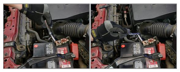
Using a correctly sized wrench or socket, loosen the nut/bolt securing the cable on the **positive** battery terminal.
