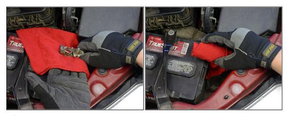
A Prevent the cable from making accidental contact with the terminal by pushing it aside and/or wrapping the cable clamp with a dry rag.
