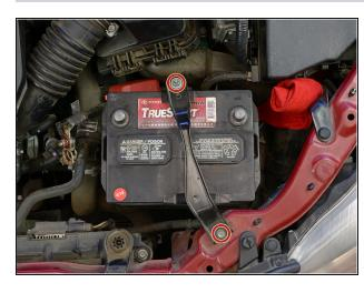
Remove any bolts securing the battery.
