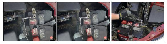
Using a correctly sized wrench or socket, loosen the nut/bolt securing the cable on the negative battery terminal.
