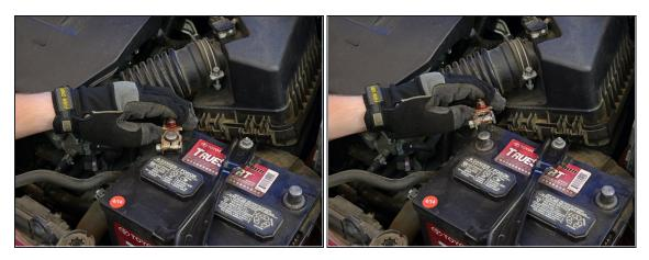
• Remove the cable from the positive battery terminal.
