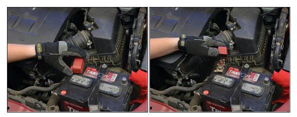
• Remove the insulating cover from the positive battery terminal (if one is present).
