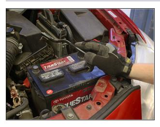
• Remove any bars or brackets securing the battery.
