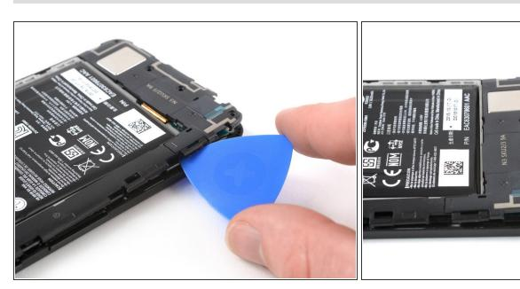
Use the plastic pick to pry open the plastic clips on the long edge of the midframe and on the bottom edge.
