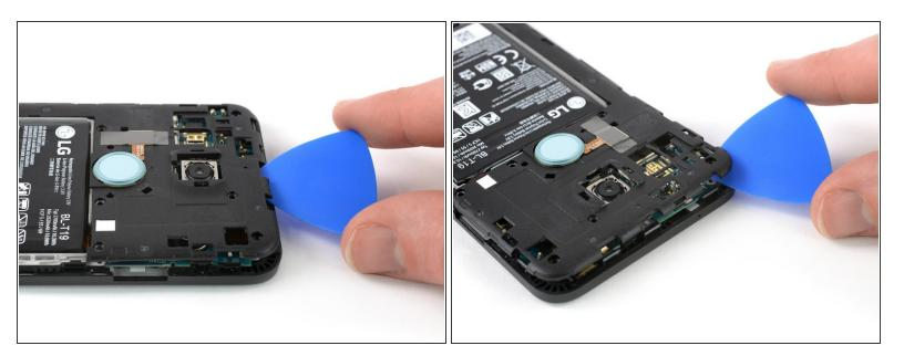
Continue sliding the opening pick around the upper part of the midframe to release the plastic clips.
