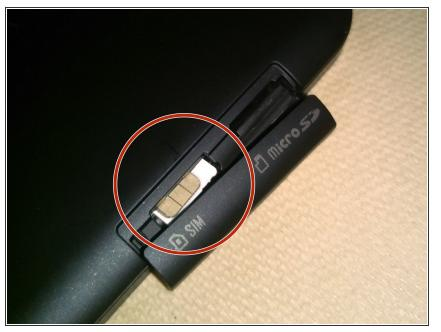
Open SIM card flap and remove SIM card. Use a pair of tweezers to get the SIM card out.
