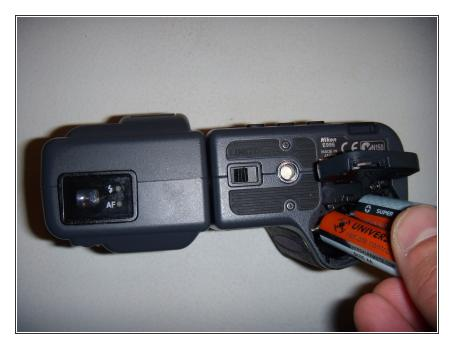
Insert the new battery as shown on the underside of the compartment lid.
