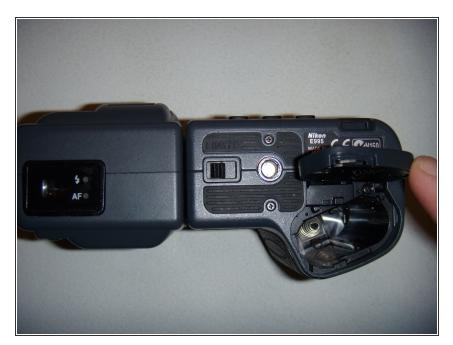
Lift the battery compartment cover and remove the old battery.
