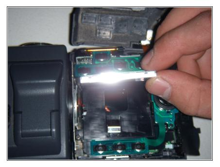
• Carefully lift the LCD from the bottom. It should come out fairly easily.
