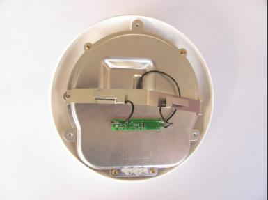
Lift the bottom and top casing straight apart and then lift metal casing straight up from the bottom plastic casing.
