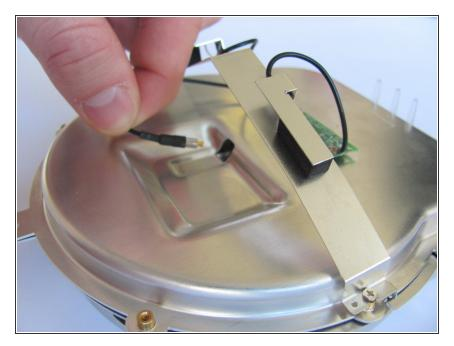
Unplug the black connector on the top of the metal casing by gently pulling horizontally.
