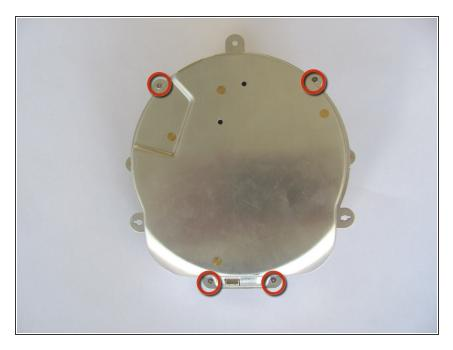
Remove the four 4.3mm phillips screws from the bottom of the metal casing.
