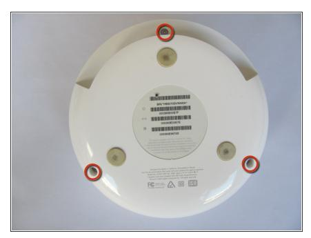
Remove the three 14.3mm T7 Torx screws from the bottom of AirPort.
