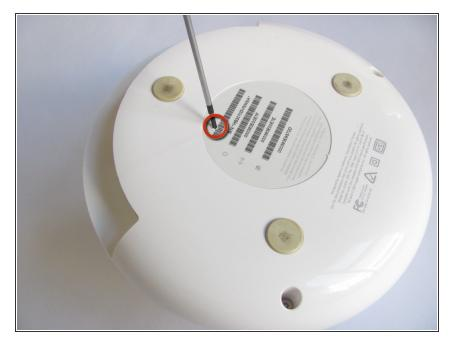
Remove the 5.1mm Phillips screw from the bottom of the AirPort. This screw is located under the identification sticker. You will have to remove the sticker or make a hole to remove it.
