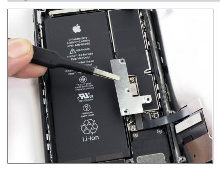
• Remove the lower connector bracket.
