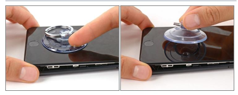
Pull up on the small nub on the suction cup to remove it from the front panel.
