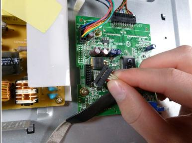
Remove the beige control cable to the left of the VGA input by pulling it up.
