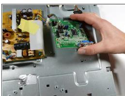
Remove the three 7.7 mm Phillips #2 screws from the motherboard, and take out the motherboard by lifting it up.
