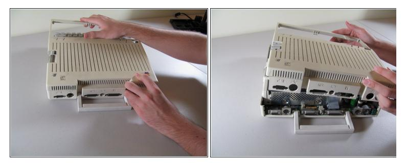
• Slide the case toward the ports on the back, then grip under the catch and pull up while moving toward the ports to remove.
