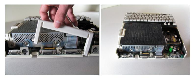
• Lift the handle straight up to remove.
