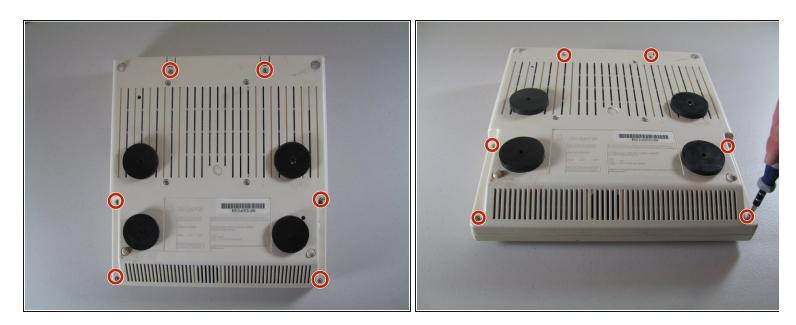
• Remove the six 19 mm long screws with a #2 Phillips head screwdriver.
