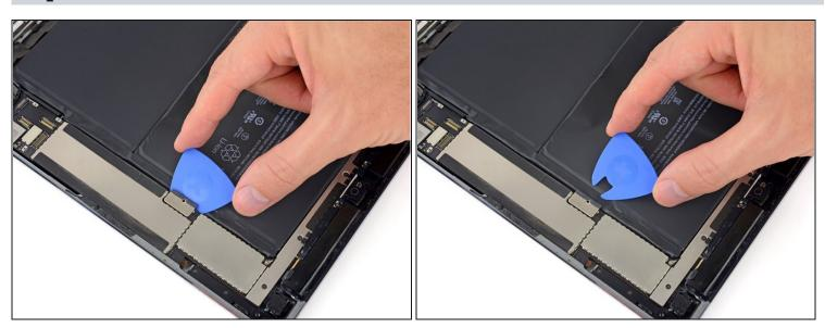
• Remove the battery isolation pick.
