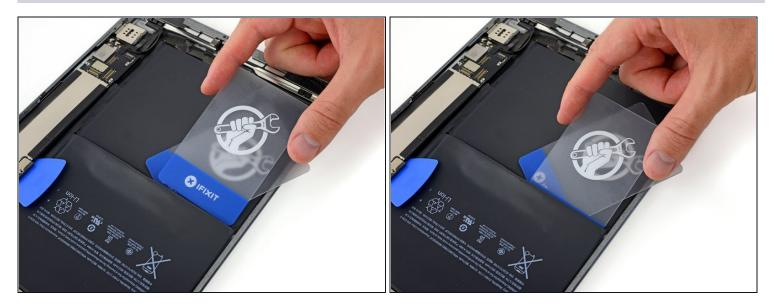
• Slide the short edge of a second plastic card underneath the battery cell and above the first plastic card.
