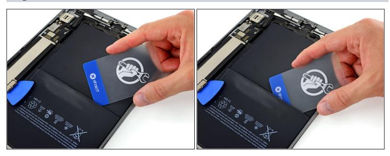
• Re-insert a corner of your plastic card under the upper battery cell, near the left edge of the iPad.
