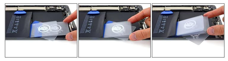
• Insert multiple additional cards *between* the first and second card to create a wedge and lever this section of the battery away from the rear case.
