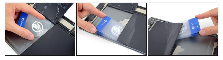
Repeat the above procedure to separate the second, lower battery cell from the rear case.
