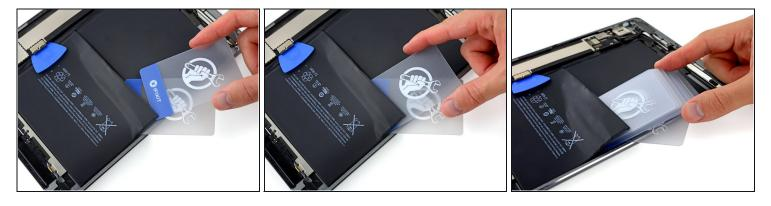
• Repeat the above steps to wedge up the lower left corner of the upper battery cell.
