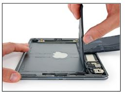
• Gently lift the lower battery cell from the edge opposite the logic board, and swing it up to separate it from the rear case.
