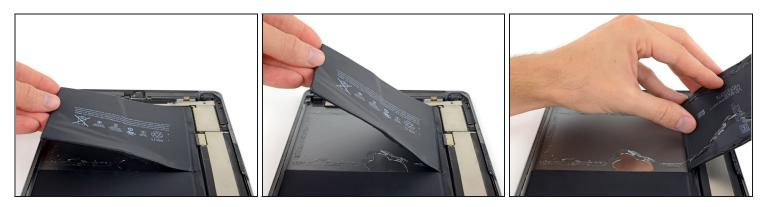
• Gently lift the upper battery cell from the edge opposite the logic board, and swing it up to separate it from the rear case.
