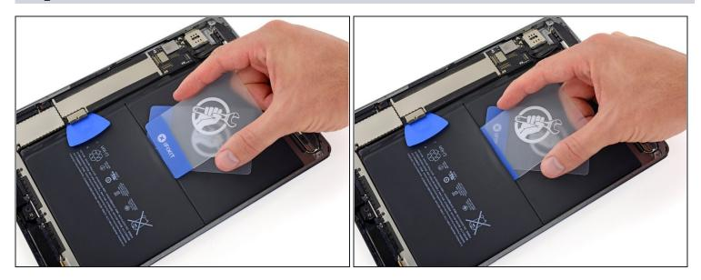
Slide the short edge of a second plastic card underneath the upper battery cell, on top
