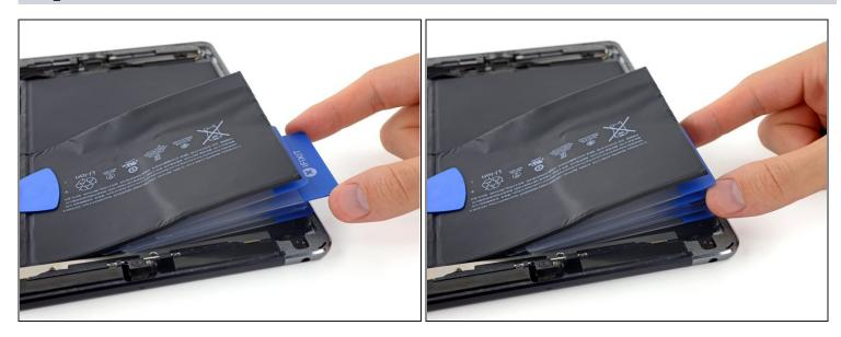
• Finish wedging up the upper battery cell using the above procedure by inserting cards along the left edge of the upper battery cell (the edge opposite the logic board).
