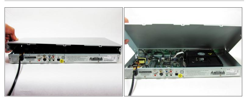
• Lift the top panel from the back and remove. It should come off without being forced. There is a lip near the front so you many need to slide the top panel back slightly to remove it.
