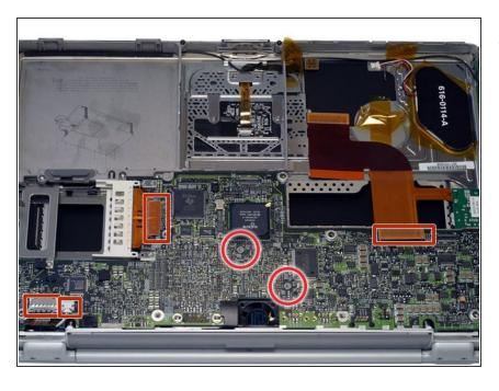
Disconnect the four indicated connectors from the logic board, removing tape as necessary.
