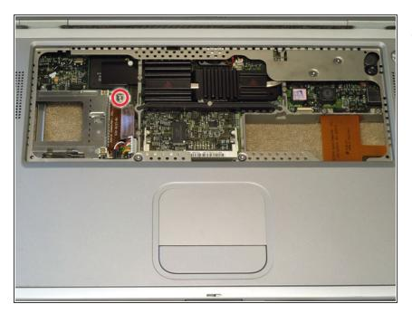
Remove the single T8 Torx screw located next to the PC Card cage.
