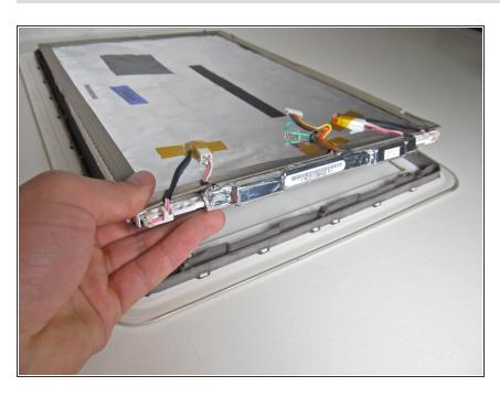
Once the four screws are removed, the display is ready to be removed and the inverter is accessible. To reassemble your device, follow these instructions in reverse order.
