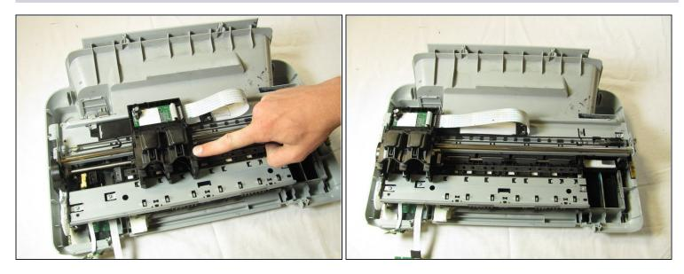
• Gently push the ink cartridge carriage to the left side of the printer.
