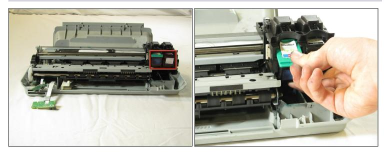
Remove both of the ink cartridges by grabbing the front of the ink cartridge and pulling down.
