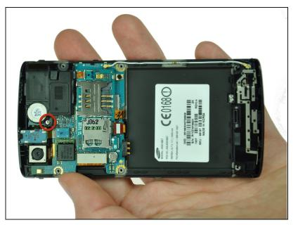
Use the Phillips 00 screwdriver to remove the single screw holding the speaker assembly to the LCD.
