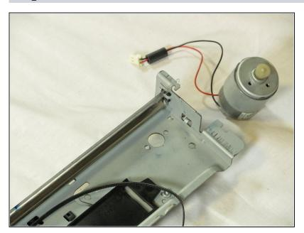
• Remove the drive motor.
