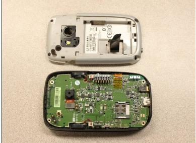
Once all the clips are open, remove the inner panel from the phone.
