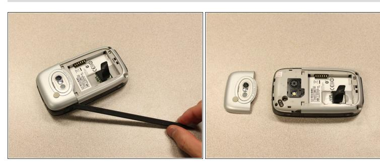
Work the <u>spudger</u> around the edges of the camera cover until it comes off.
