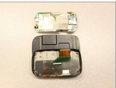
Remove the flexible connection from the motherboard.
