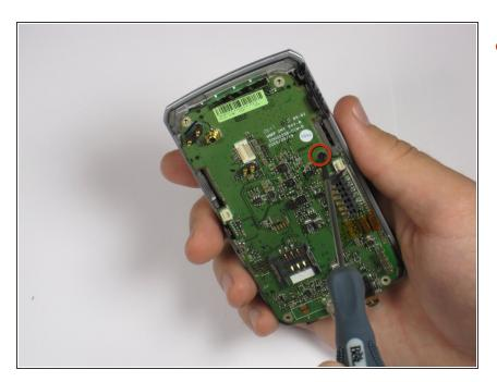
Remove the 3.4 mm black screw with the Phillips #000 screwdriver.
