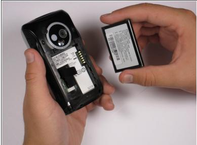
Pull on the plastic tab to release the battery.
