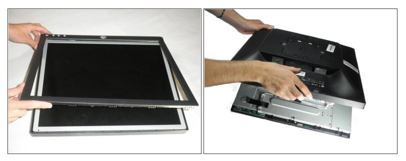
• When finished prying, the plastic will partially fall away from the rest of the monitor.
