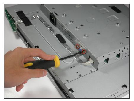
Using a 5 mm nut driver, unscrew the VGA port's mounting screws from the metal casing.
