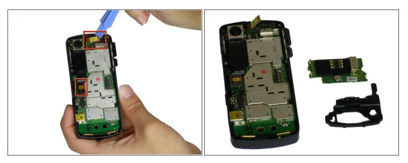
Use a plastic opening tool to pry the two ribbon cable connectors, unclipping them from their sockets on the motherboard.
