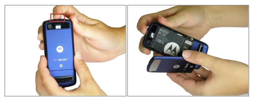
Press the panel release button on the top of the phone and simultaneously pull the rear panel away from the phone.
