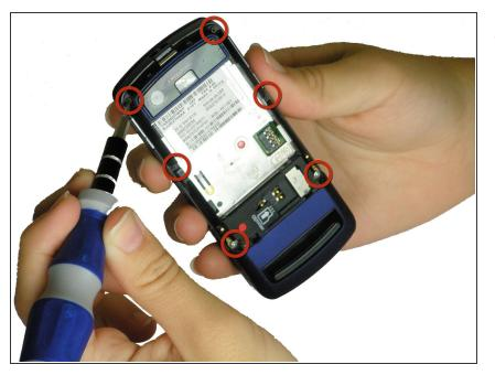
Use a T4 screwdriver to unscrew all six of the .216 inch screws that attach the housing to the case.
