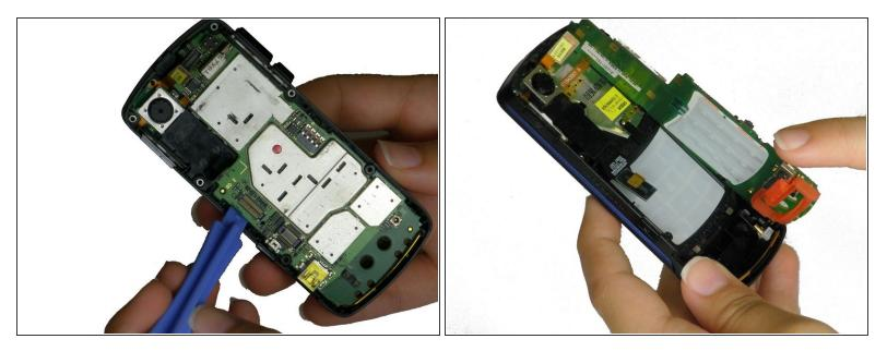
• Use a plastic opening tool to gently pry the motherboard up until you can tilt it with your fingers. Unhook it from the casing and slowly pull it out.
