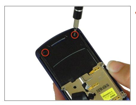
• Use a T4 screwdriver to unscrew the two .15 inch screws holding the LCD to the faceplate.
