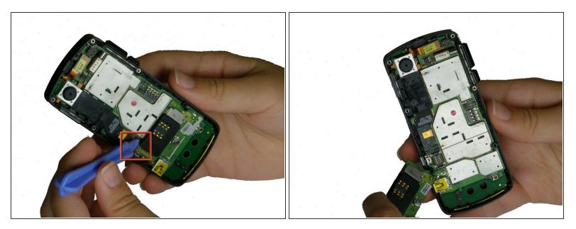
Use a plastic opening tool to gently lift up the SIM card reader, located above the rubber antenna casing. You should hear a click as it releases.
