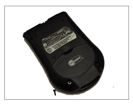
Place the battery door back into place on the back of the device; it will make a 'click' sound when properly reattached.
