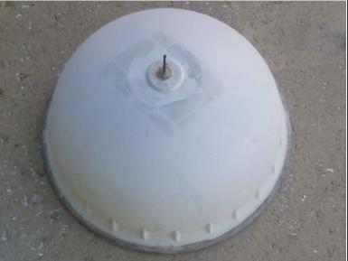
Remove the top half of the filter housing.
