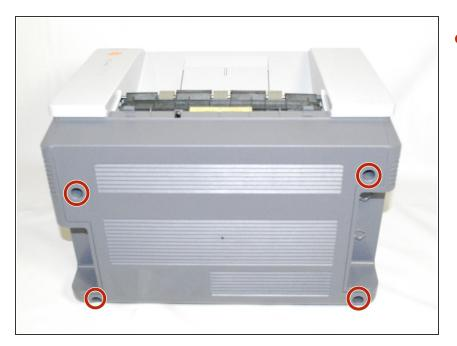
Using a Phillips #2 screwdriver, remove the four screws on the back of the printer.
