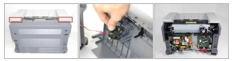
• Gently lift the top panel while simultaneously pulling off the back panel.
