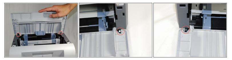
• Remove the front panel by gently moving the holes on the panel, one at a time, from the pegs attached to the main body of the printer.
