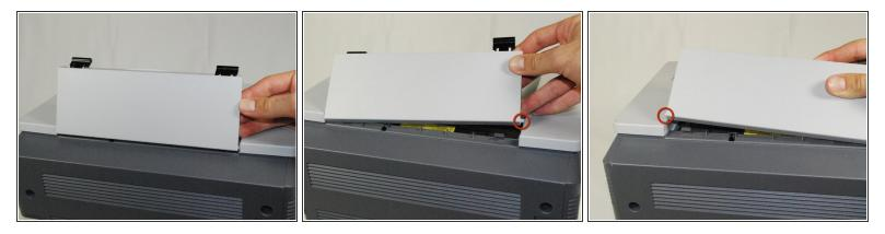
• Remove the top hinged panel by taking out the pins at the bottom of this panel.
