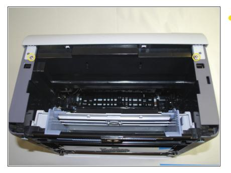
Use a Phillips #2 screwdriver to remove the two, 1", Phillips, PH#2 screws on the front face of the printer.
