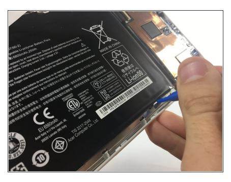
Use the plastic opening tool to gently wedge out and lift the battery pack from the device.
