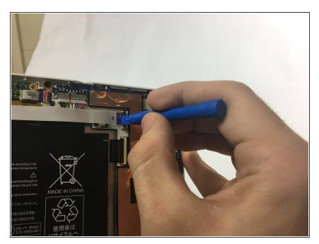
Pull the ribbon cord by pushing the clamp on the port toward you with the plastic opening tool.
