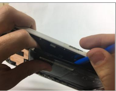
Carefully break the bond between the inner tape and the battery using the plastic opening tool. The tape can be found in the middle and either side of the battery.
