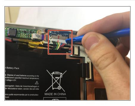
Use the plastic opening tool to carefully slide the power cord from its slot by pushing it out from both sides, then remove the cord from its port with your hand.
