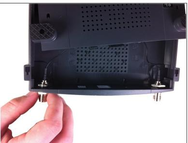
Unscrew the nut on the outer side of the back casing. Remove the nut and the washer from both antenna mounts.
