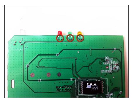
Place new LED lights through holes created by desoldering and removing old lights.
