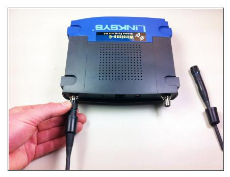
Remove the antennas from the back of the device. To do this, follow steps 1 and 2 of Installing the Antennas Guide: <u>Linksys WAP54g</u> <u>Antennas Replacement</u>
