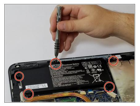
Remove the five 6mm screws that hold the battery in place using the Phillips #0.
