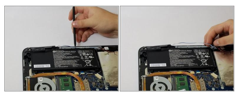
• Use the nylon spudger to pry away the blue/white wire that is positioned near your battery.
