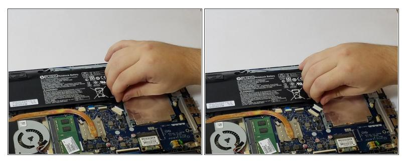
• Disconnect the battery cable from the motherboard by carefully pulling on the black wire at the point closest to the white tab.
