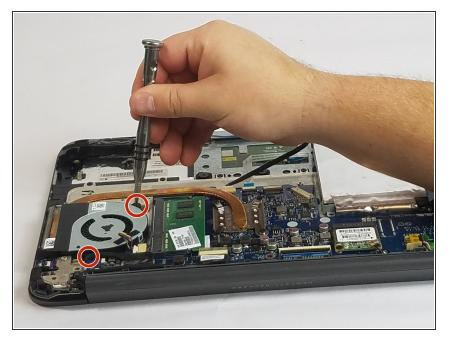
Use the Phillips #0 to remove the two 3mm screws holding the fan in place.
