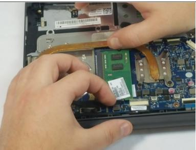
Using your fingernails, pull the tabs on either side of the RAM to release the module from its secured spot.
