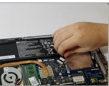
Disconnect the battery cable from the motherboard by carefully pulling on the black wire at the point closest to the white tab.
