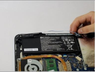
• Use the nylon spudger to pry away the blue/white wire that is positioned near your battery.
