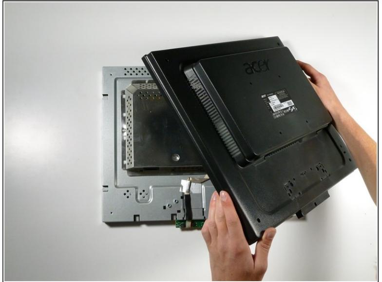
**i** Reposition the monitor so that the back is facing up.
