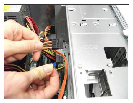
• Disconnect the two cables from the back of the hard drive.
