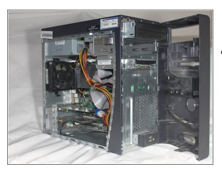
Swing the front of the case open until it separates from the main case.
