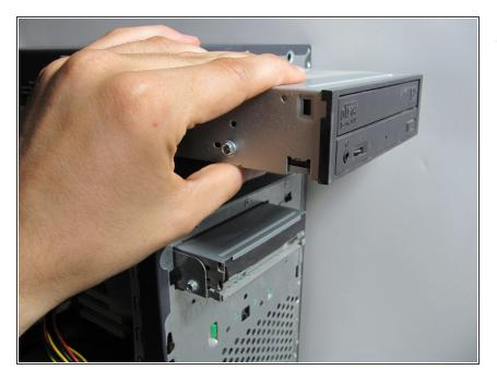
• Remove the optical drive by sliding it out of the front of the case.
