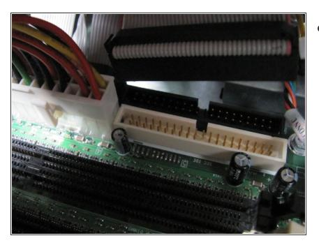
Grasp the end of the Drive 1 cable connected to the motherboard and firmly pull upwards until it is removed.
