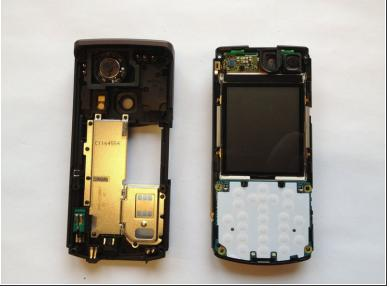
• Separate the front panel of the phone by pulling the bottom of the panel at a 45 degree angle.
