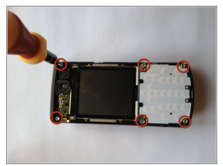
Using a torx T6 screwdriver remove the six 15 mm torx screws.
