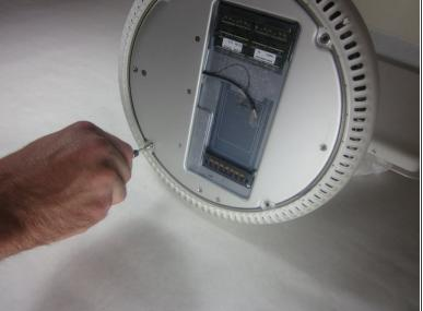
Remove the four 25mm T-15 screws.
