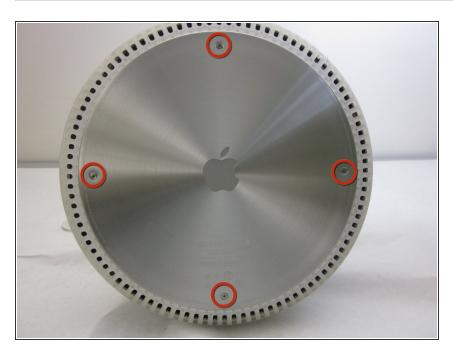
Loosen the four Phillips #0 screws.
