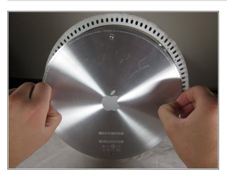
Carefully remove the base access panel.
