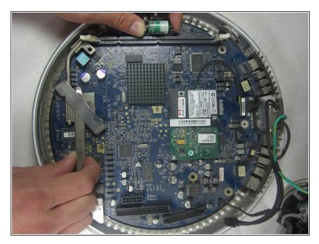
Using thumbs and forefingers, firmly grasp the battery holder in one hand while grasping the metal bar in the other. Gently lift and pull the logic board to release it.
