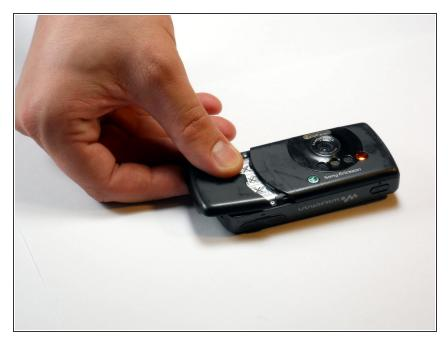
Remove the battery cover by applying downward pressure on the Singular Symbol and then shifting the pressure towards the bottom edge of the phone.
