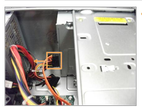
Locate and remove the two cables attached to the CD/DVD drive.
