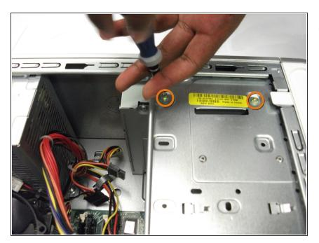
Locate and remove the two Phillips #0 7.8 mm screws.
