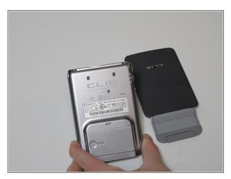
After unlocking the cover slide lock, remove the cover and set aside.
