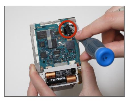
Using a Phillips #0 screwdriver, remove the two screws holding the scroll wheel in place.
