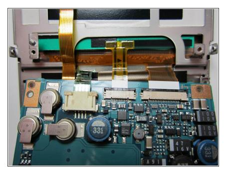
Rotate the motherboard 180 degrees so that it is upside down facing toward you to expose the power cables on the other side.
