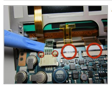
Gently pull out the clips to remove the top power cables from the motherboard.
