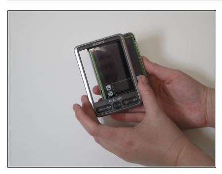
Remove the front case by gently lifting away from the device.
