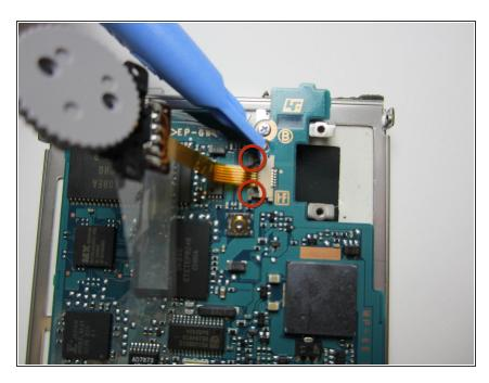
Pull out both sides of the clip to remove the scroll wheel power cable from the device.
