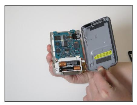
Gently pry off the right side off the back panel and set it aside, leaving room for the scroll wheel at the upper right corner.
