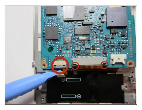
Gently pull out the clips to remove the bottom power cables from the motherboard after removing the battery harness.
