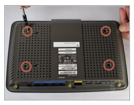
Remove the 0.4cm head screws from each slot with the #1 Phillips head Screwdriver.
