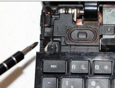
Use a Phillips #1 screwdriver to remove the two 7mm screws located on either side of the keyboard panel.
