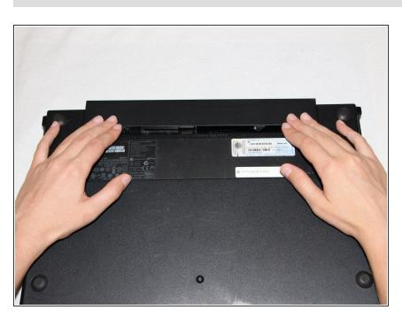
Remove the battery by holding the latches and sliding the battery away from you.
