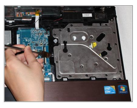
Use a metal spudger to push the optical drive to the right and partially out of the casing.
