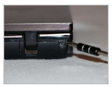
Use a Phillips #1 screwdriver to remove the 3mm screws behind the caps.
