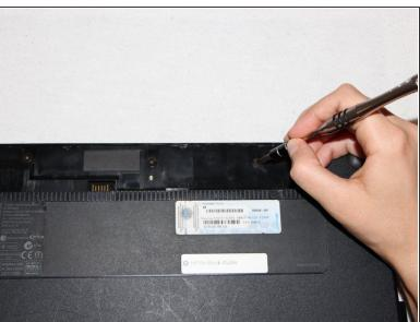
Use a Phillips #1 screwdriver to remove three 2mm screws where the battery was located.
