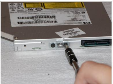
Use a Phillips (PH1) head screwdriver to remove two 2mm screws securing the metal tab to the optical drive.
