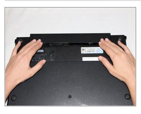
Remove the battery by holding the latches and sliding the battery away from you. To reassemble your device, follow these instructions in reverse order.
