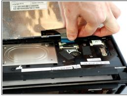
• Locate the sticker-like connecter on the back of the keyboard. Carefully unplug it.
