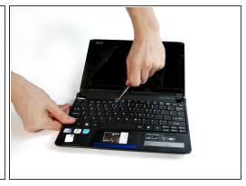
Using the metal spudger, gently pry each tab releasing the keyboard. Make sure as you move to each new one that the previous one does not reset itself.
