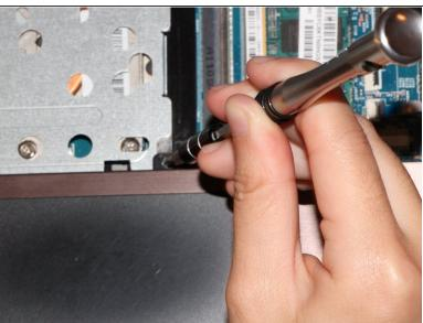
Use a Phillips #1 screwdriver to remove the three 3mm screws along the top of the palm rest.
