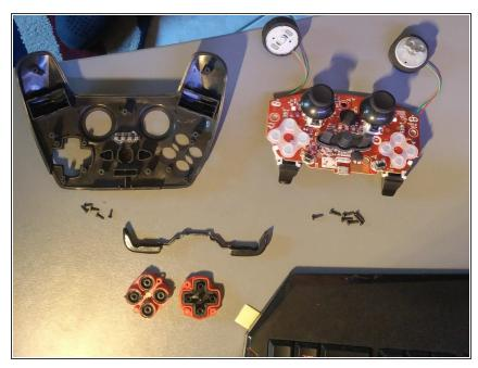
(i) You now have a fully disassembled controller, ready to be repaired or modified
