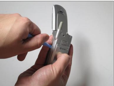
Wedge the opening device into the side crease of the phone.
