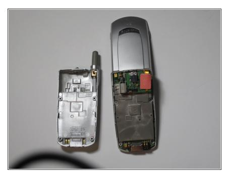
Remove the back casing from the front casing. Force may be necessary.
