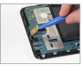
Disconnect the wire near the top of the motherboard by placing the plastic opening tool under the edge of the connector to flip it up.
