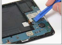
Disconnect the wire near the bottom of the motherboard by placing the plastic opening tool under the edge of the connector to flip it up.
