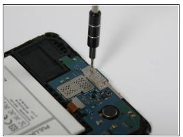
Using a Phillips #00 Screwdriver, remove the five 4 mm screws connecting the motherboard to the frame of the device.
