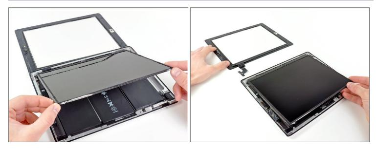
In order to remove the front panel assembly, the ribbon cable needs to slide out between the case and the LCD. You'll need to move the LCD to make some room.
