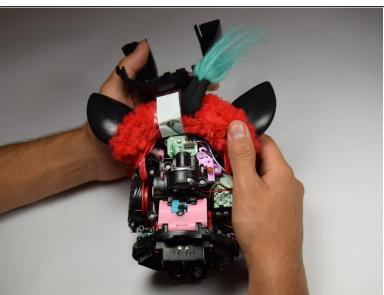
Remove the loose, plastic back panel by pulling the panel away from Furby's body.
