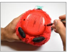
Use a flathead screwdriver to remove the two 10mm screws on the base of the Furby.
