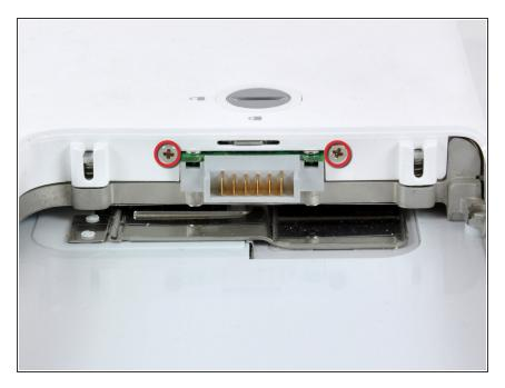
Remove the two Phillips screws on either side of the battery contacts.
