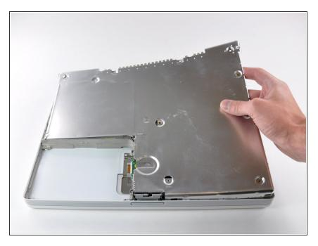
Lift the bottom shield off.
