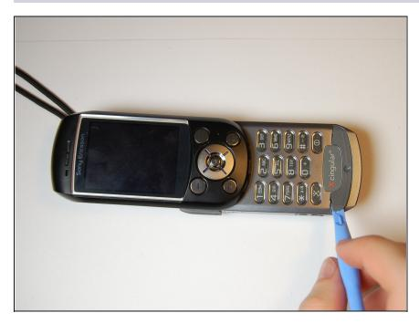
• Remove the microphone cover using the iFixit opening tool.
