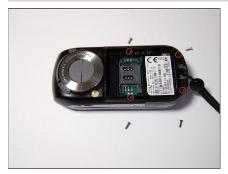
• Remove the four 6 mm screws from beneath the battery using a Phillips #00 screwdriver.
