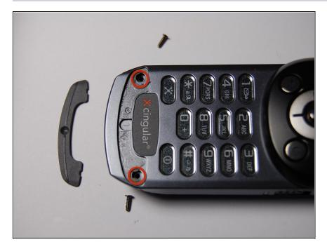
Remove the two 6 mm screws from the front of the phone beneath the microphone cover using a Phillips #00 screwdriver.
