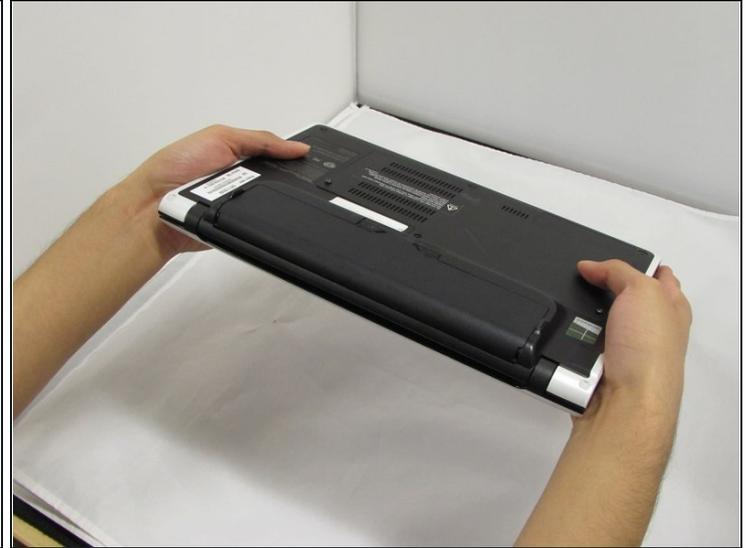
**⚠ Remove the charging adaptor. Some charge may still be in the battery or computer. DO NOT touch connectors or copper yellow connector.**
